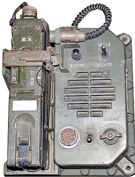
RR-117 receiver (left) and AD-112 vehicle cradle (right).
