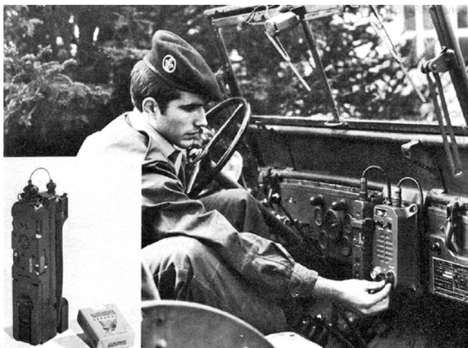
RR-VP 5 station fitted in a French M 201 Hotchkiss jeep.
